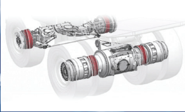
Front and rear wet disc brakes
